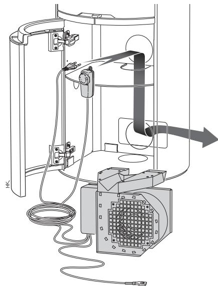
Thread the control box and the plug through the rear panels.
