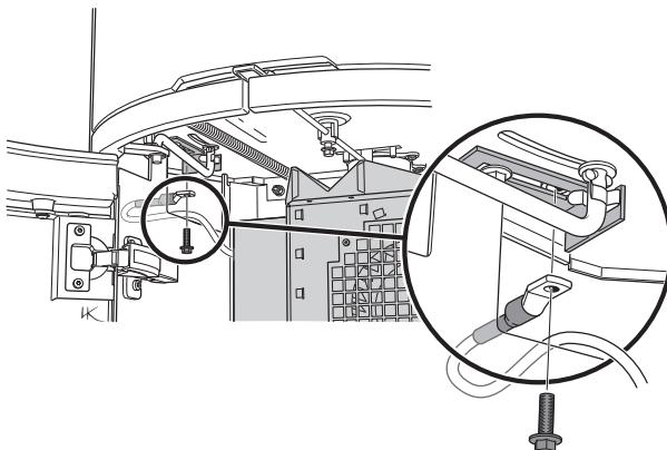
Remove the inner screw on the plate at the grate control. Secure the temperature sensor in the hole using the M6X20 screw supplied.
