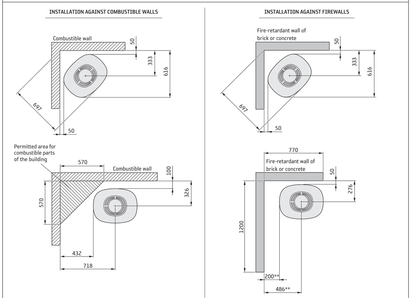
\* If the stove is placed on a hearth plate made of glass for example (accessory), the height from the floor is affected by a distance corresponding to the thickness of the hearth plate, for a free standing glass hearth plate this is 10 mm.
