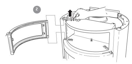
Hold the oven door in place on the threaded pin. Hook the top hinge in place and loosely tighten one of the screws. Close the oven door and adjust it so that it aligns horizontally. Then open it carefully and tighten both screws.
