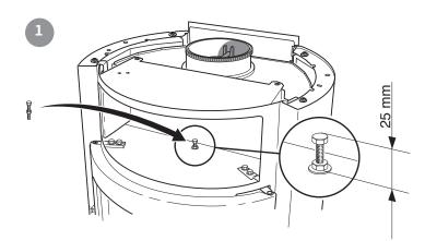
Replace the preinstalled adjuster screw in the heating compartment with the longer adjuster screws provided. Place the warming shelf in the heating compartment, use the adjuster screw at the rear edge for horizontal installation. In the side of the heating compartment there is a small gap, this is used to install the rear cover panel.
