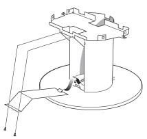
There is a detachable cover on the reverse of the pillar foot which is removed when installing combustion air connection.
