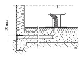
Through floor and foundation slab.
