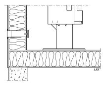
Indirect air supply through the external wall.
