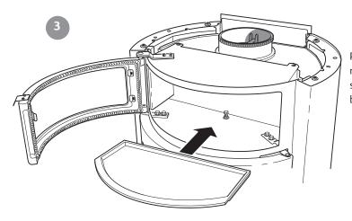
Place the baking sheet in the oven. If necessary, adjust the height of the baking sheet by turning the adjusting screw at the bottom of the oven unit.
