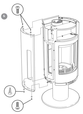
Adjust the side panels so that they are against the insert and so that there is an even join against the back plate.
