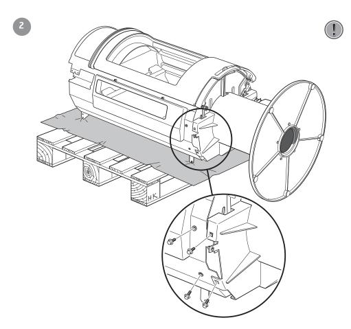
The pillar is mounted using four screws. The remaining four screws must also be reinstalled to prevent air leakage into the firebox.
