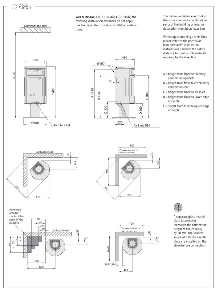
If the stove is placed on a hearth plate made of glass for example (accessory), the height from the floor is affected by a distance corresponding to the thickness of the hearth plate. Also applies to separate glass hearth plates (accessory).
