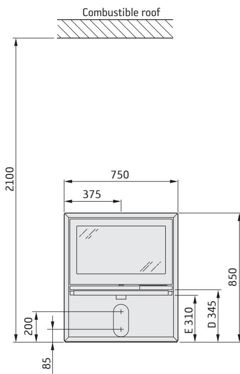
The minimum distance in front of the stove opening to combustible parts of the building or interior decoration must be at least 1,4 m.
