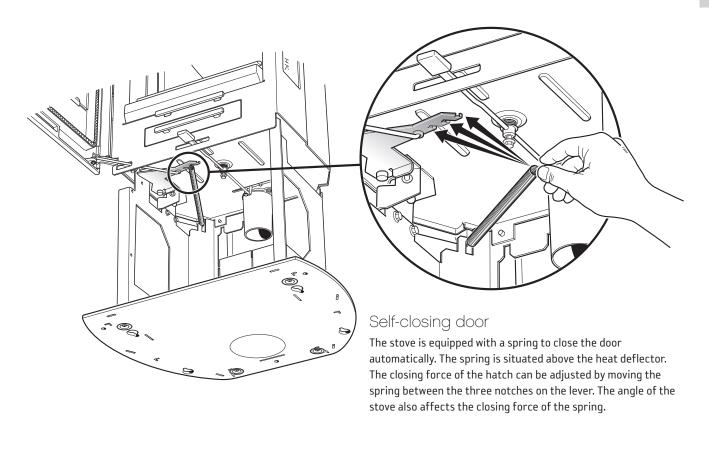
If the spring force seems weak, despite the spring being mounted at the end of the lever, the angle of the stove should be checked. Adjust with adjustable feet if necessary.
