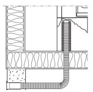
In the case of connection through the floor, first remove the knockout in the guide plate and any hearth plate.
