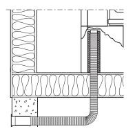
In the case of connection through the floor, first remove the knockout in the guide plate and any hearth plate.
