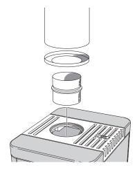
Make sure that the connector gasket does not come loose when the connection pipe is placed on the sleeve. If further sealing material is required, heatresistant sealant may be used.
