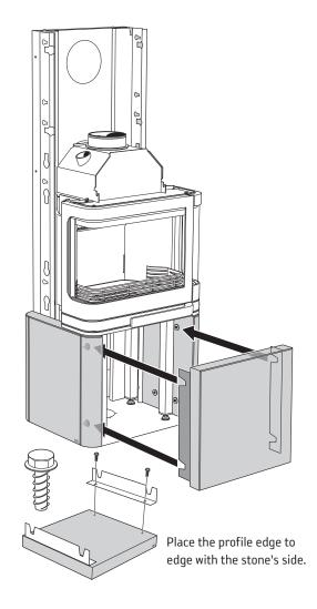
Wait to tighten this screw until the next stone is in place.
