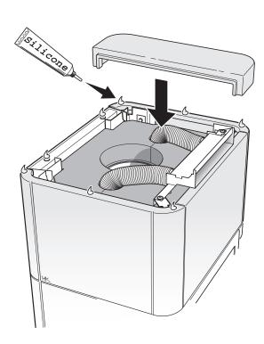
Ensure that joints are clean and dry before applying the sealant.
