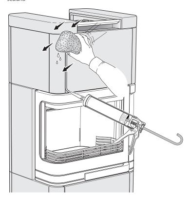
Work the sealant in with a lightly dampened sponge in diagonal movements. After the sealant has dried the tiles can be wiped clean.
