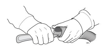
Open and fold out any deformed edges in the pipe opening to facilitate installation.
