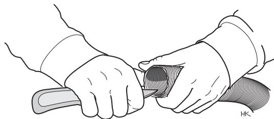
Open and fold out any deformed edges in the pipe opening to facilitate installation.
