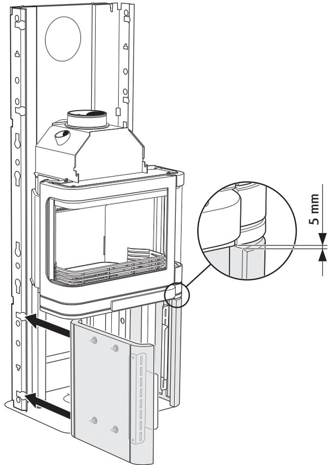
Place the profile edge to edge with the tile's side.
