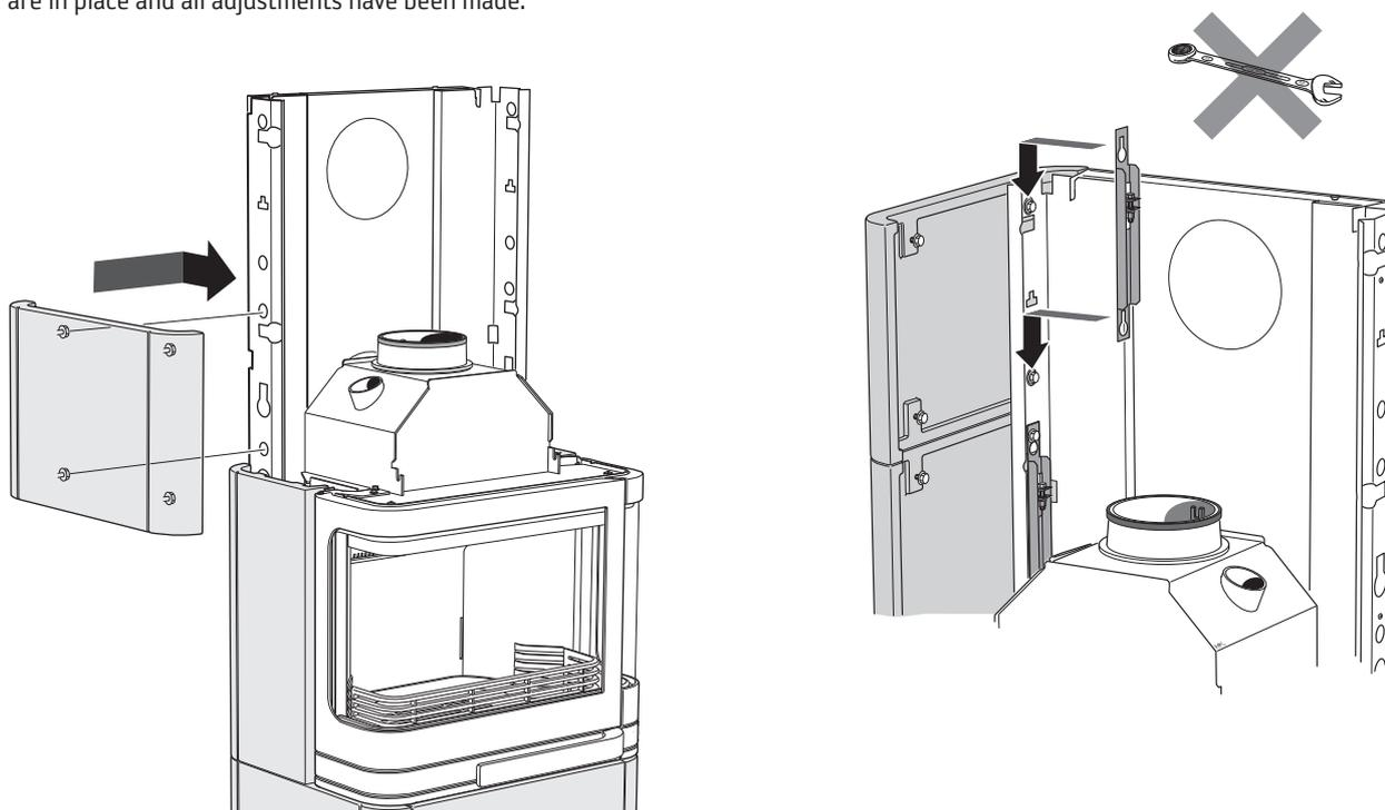
Prevent the side panels from dipping forward by hooking the hooks in the rear profile and tightening the screws until they engage
