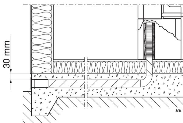
In the case of connection through the floor, first remove the knockout in the guide plate and any hearth plate.
