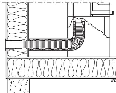
For this type of connection, first remove the valance that sits in front of the back plate's air intake.
