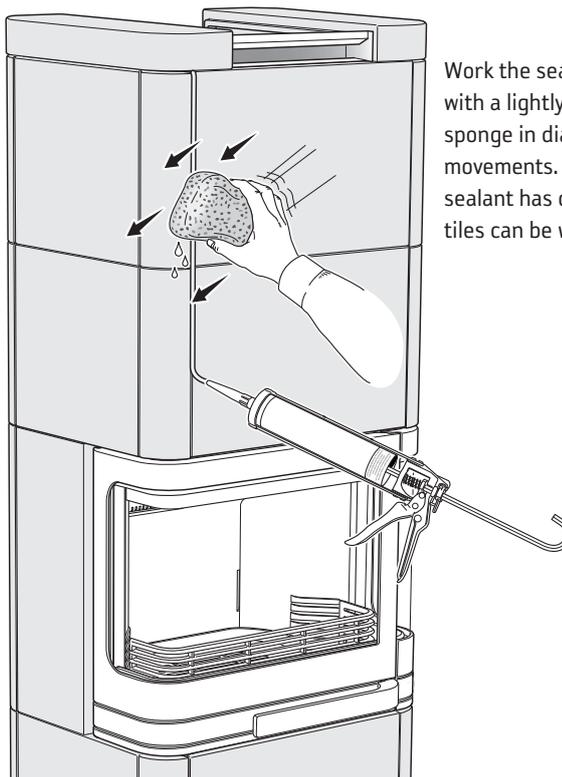
Work the sealant in with a lightly dampened sponge in diagonal movements. After the sealant has dried the tiles can be wiped clean.
