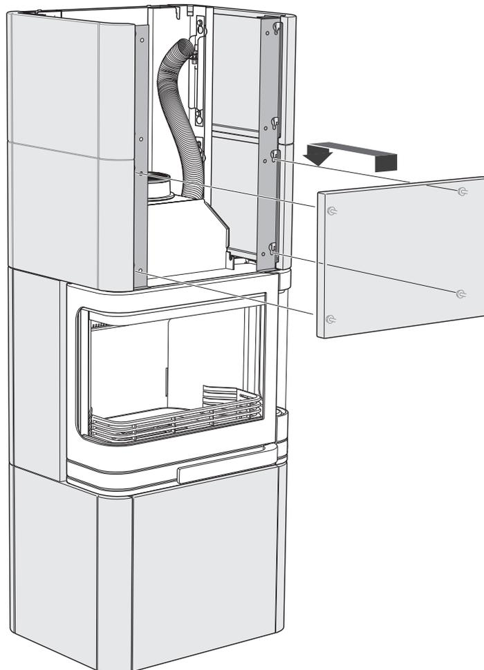
The front plates are moved up slightly by hooking the hooks in the rear profile and tightening the screws. Tighten the screws until the upper plates align with the upper edge.
