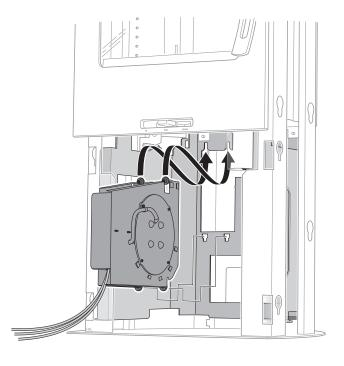
Angle the lower silicone cones into the leg's lower cut-out.
