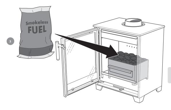
Add briquetts on top of the glowing embers, about 0,6-0,7 kg and close the door.
