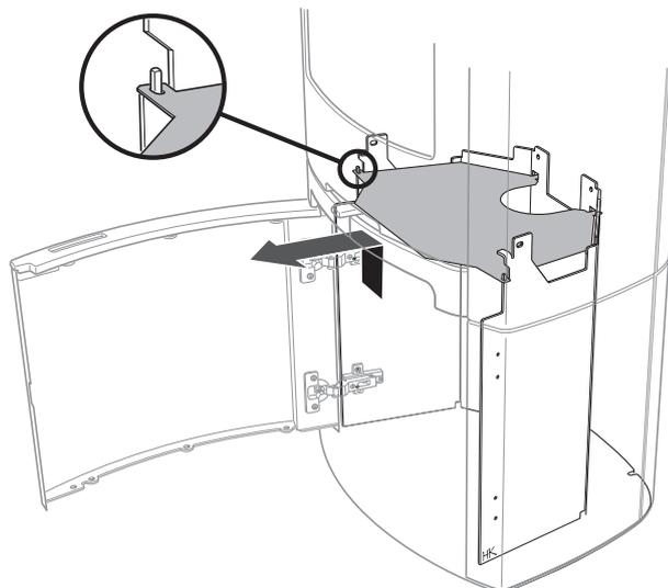
How to remove the firebricks
