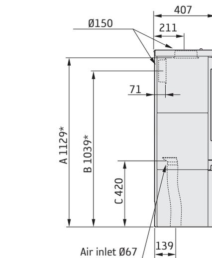
The minimum distance in front of the stove opening to combustible parts of the building or interior decoration must be at least 1 m.
