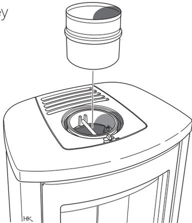
**!** Make sure that the connector gasket does not work loose when the connection pipe is placed on the connector. If further sealing material is required, heat-resistant sealant may be used.
