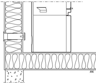
Indirect air supply through the external wall.
