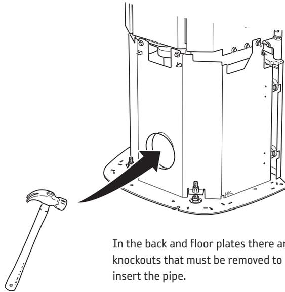
In the back and floor plates there are knockouts that must be removed to insert the pipe.
