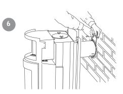
Make sure that the connector gasket does not work loose when the connection pipe is placed on the connector. If further sealing material is required, heatresistant sealant may be used.
