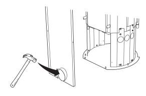
In the back and floor plates there are knockouts that must be removed to insert pipes or for air supply if the stove is equipped with a lower hatch and/or fan (accessory).
