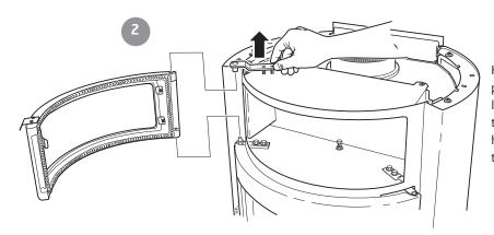
Hold the oven door in place on the threaded pin. Hook the top hinge in place and loosely tighten one of the screws. Close the oven door and adjust it so that it aligns horizontally. Then open it carefully and tighten both screws.
