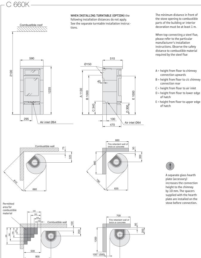
\* If the stove is placed on a hearth plate made of glass for example (accessory), the height from the floor is affected by a distance corresponding to the thickness of the hearth plate. Also applies to separate glass hearth plates (accessory).
