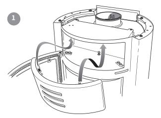
Open the hatch and install the convector fascia with the retaining brackets angled as shown.
