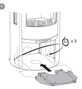
Slacken off the rear Allen screws three turns. Place the pull-out unit on the base plate.
