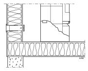
Indirect air supply through the external wall.
