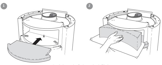
Place the bottom plate for the warming shelf in the heating compartment, use the adjuster screw at the rear edge for level horizontal installation. Place paper from the packaging as scratch protection because the upper section must be slid into position.
