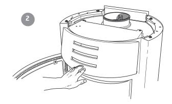
Insert the convection fascia upwards first so that the locking spring comes inside the front panel of the stove and push the convection fascia lightly upwards. Then press the fascia in and allow it to slide into place.
