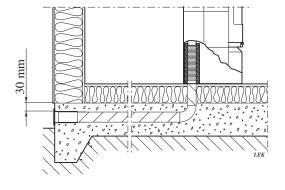
Through floor and foundation slab.
