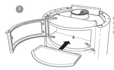
Place the baking sheet in the oven. If necessary, adjust the height of the baking sheet by turning the adjusting screw at the bottom of the oven unit.
