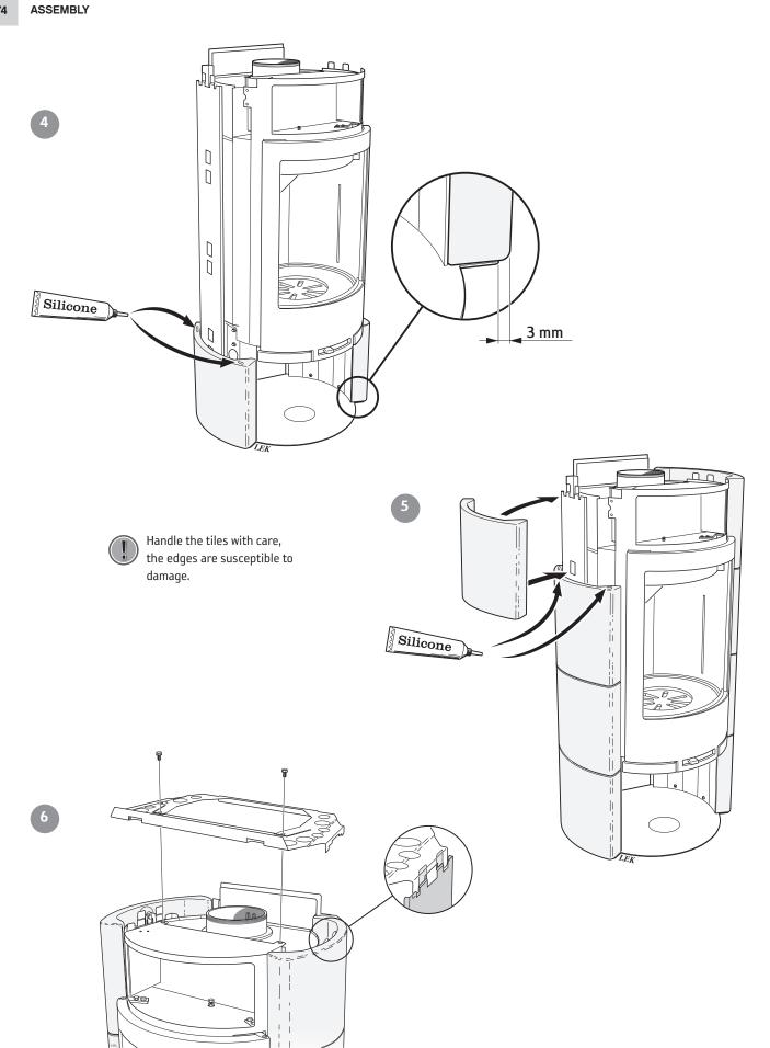
Install the convection fascia, warming shelf or baking oven according to the instructions in the section for the relevant accessory on pages 76 to 77. This must be done before the tiled top is installed.
