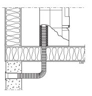
Through floor and wall-and-cavity foundation.
