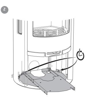
Hook the pull-out unit into place over the rear Allen screws. Screw the unit into place.
