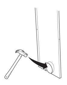
When installing the drawer, the knockout in the back panel must always be removed for the supply of convection air.
