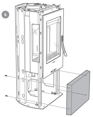
If a fan is to be installed, it has to be done before the lower front stone is put in place.
