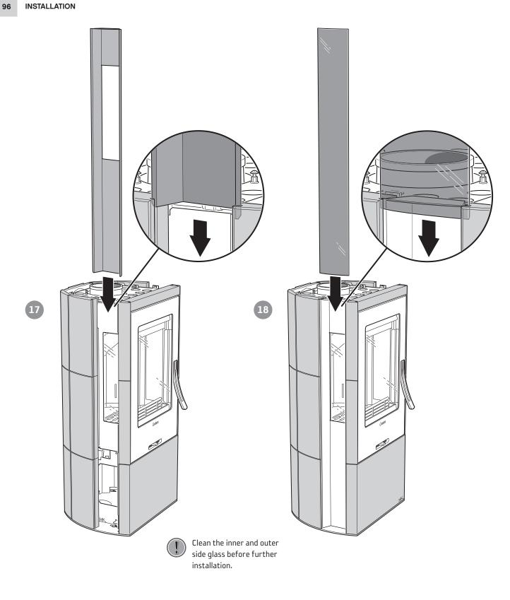
Carefully insert the profile and glass and move down the groove.
