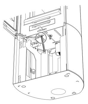
If the spring force seems weak, despite the spring being mounted at the end of the lever, the angle of the stove should be checked. Adjust with adjustable feet if necessary.
