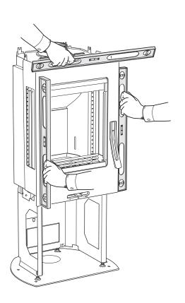
If the spring force seems weak, despite the spring being mounted at the end of the lever, the angle of the stove should be checked. Adjust with adjustable feet if necessary.
