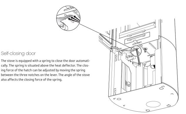
If the spring force seems weak, despite the spring being mounted at the end of the lever, the angle of the stove should be checked.
