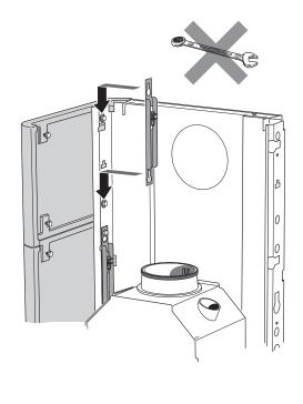
Prevent the side panels from dipping forward by hooking the hooks in the rear profile and tightening the screws until they engage
