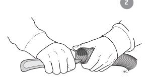
Open and fold out any deformed edges in the pipe opening to facilitate installation.
