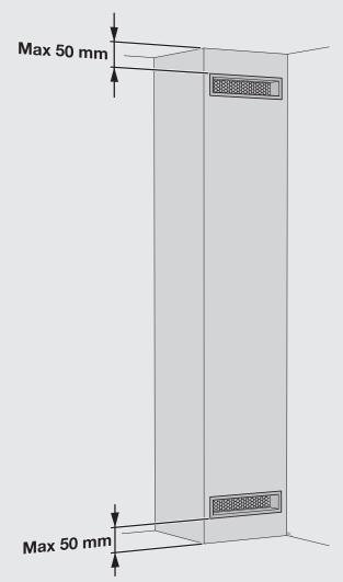
In multi occupancy residences, the shaft must satisfy the requirements that are stipulated for fire cells. Rating El60 in a fire cell boundary is achieved by integrating the chimney in an unventilated shaft comprising 50 mm calcium boards.
