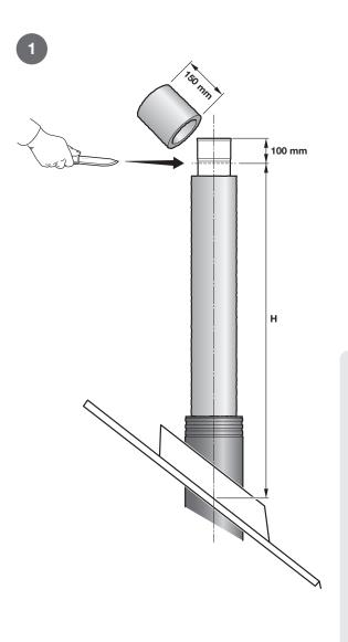
The length of the cowl jacket is established by measuring the distance from the end of the flue down to the upper plate and reducing the measurement by 100 mm (H-measurement).
