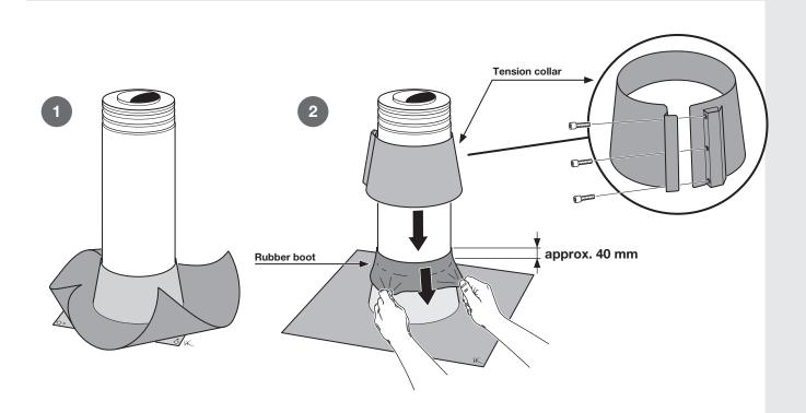
To make it easier to install the rubber boot, soap can be applied to the jacket.
