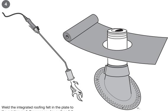
Weld the integrated roofing felt in the plate to the existing roof. If necessary, lay surface felt over the plate roofing felt and up to the ridge.
