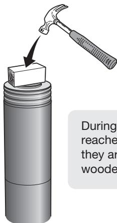
During installation, ensure that the flue pipe reaches the bottom of the connection when they are joined by tapping gently with a wooden block.
